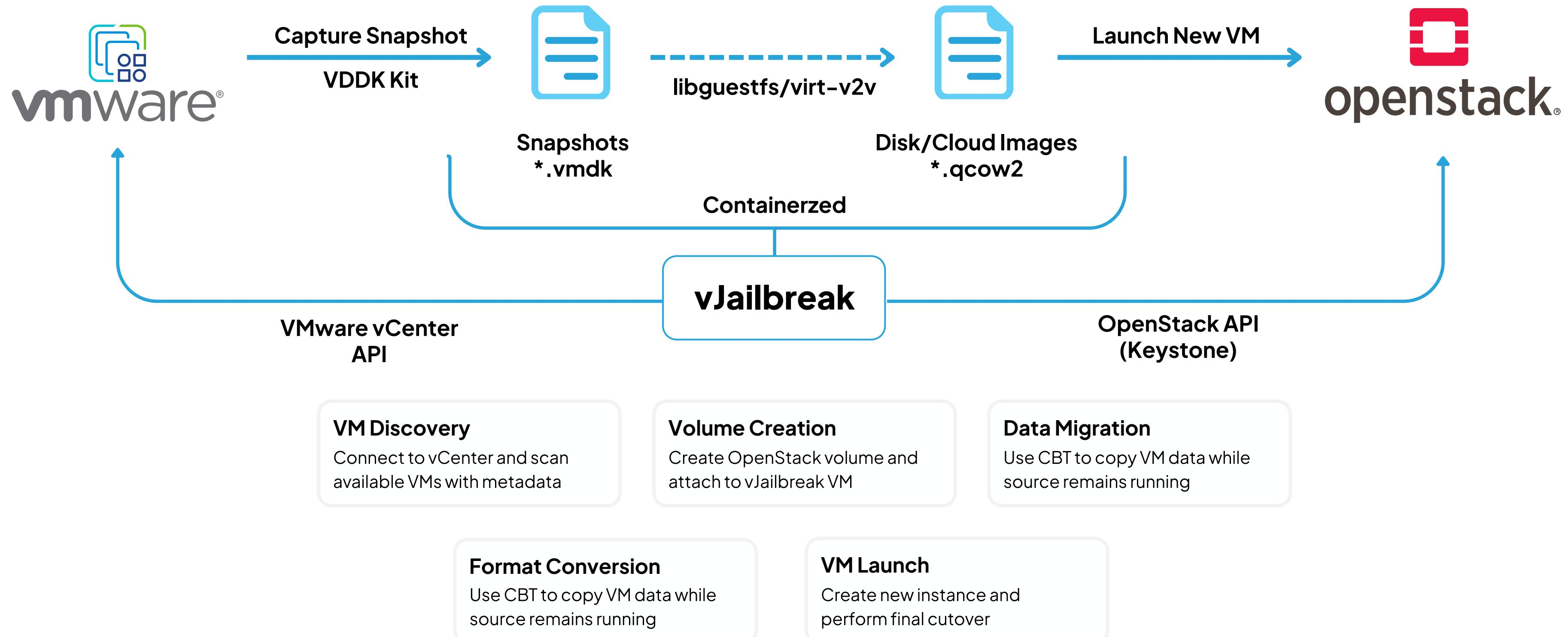
This architecture enables live migration with minimal downtime by leveraging Changed Block Tracking during the data copy phase, while the containerized conversion process ensures consistent and reliable format transformation from VMware VMDK to OpenStack-compatible QCOW2 format.
